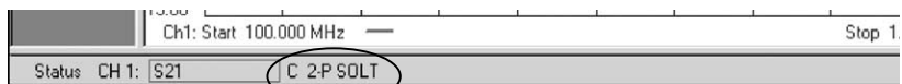
Figure 5. The MW PNA status bar provides you with valuable information, including the calibration type and status.
